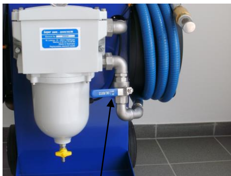
Shut-off valve closed
