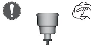
Clean container and drain valve
